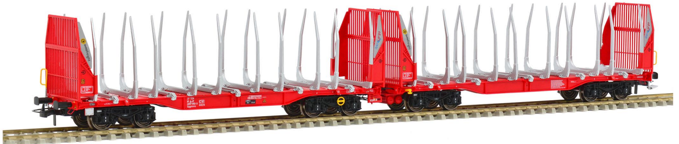
S657002 Ibercargo articulated double timber transport wagon Sggmrrs | Vagão articulado duplo transp. madeira Ibercargo Sggmrrs - A-IF 37 81 4657 002-3
